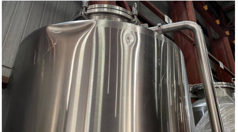
5bbl number5 shape changed on the top few more scratch on the surface
