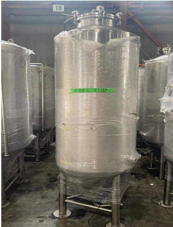
5bbl number 1 scratch on the top surface
