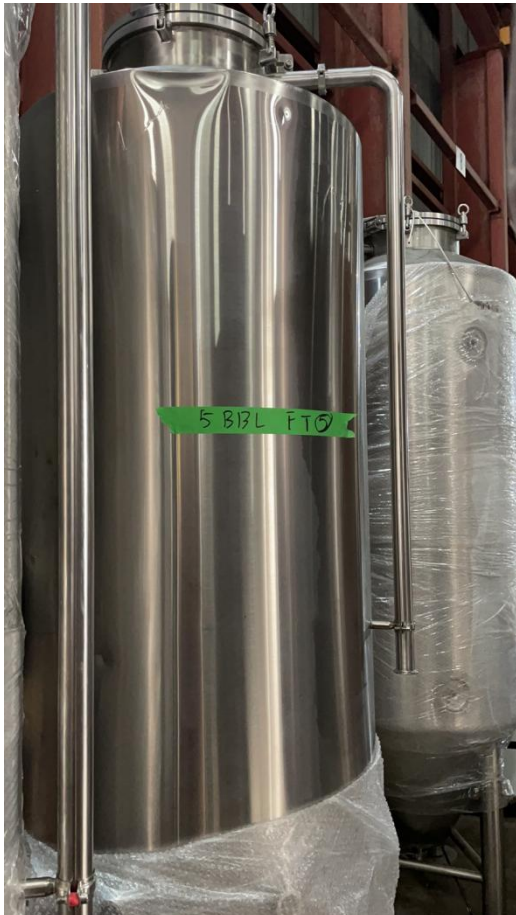
5bbl number5 shape changed on the top few more scratch on the surface
